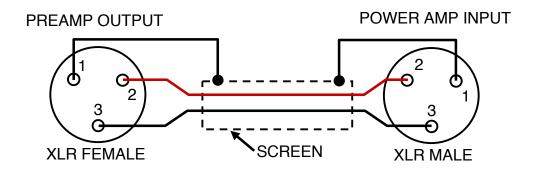
**CONVENTIONAL: SCREEN CONNECTED AT BOTH ENDS**
