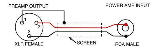
CABLE CONFIGURATION FOR XLR BALANCED PREAMP
