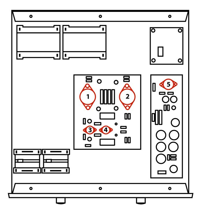
VALVE 1: 300B VALVE 2: 300B VALVE 3: 5687 VALVE 4: CV4068 VALVE 5: 5U4GB
