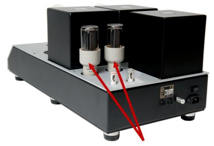
Looking from the back of the amplifier, insert the **5R4WGB** valves into the two empty sockets located on the left, situated between the black rectangular transformer covers and the loudspeaker connection binding posts. Locate the rib on the central pin of the valve and align with the valve base (it can only be inserted one way due to this locating rib) and with gentle but firm pressure insert the valve.
