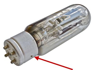
Inspect a 211 valve and you will notice that there is a small 'pin' protruding from one side of the valve base; this locating pin ensures that the valve can only be correctly inserted into the amplifier in one way.
