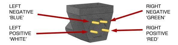
UNDER NO CIRCUMSTANCES SHOULD THE HEAD-SHELL WIRES BE SOLDERED DIRECTLY TO THE CONNECTION PINS OF THE CARTRIDGE BODY. HEAT APPLIED TO THE CONNECTION PINS WILL CAUSE IRREPARABLE DAMAGE.
