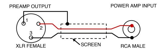
CABLE CONFIGURATION FOR XLR BALANCED PREAMP
