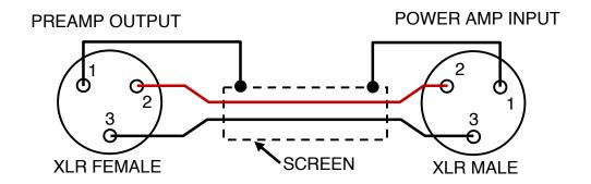
**CONVENTIONAL: SCREEN CONNECTED AT BOTH ENDS**
