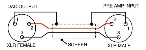
**CONVENTIONAL: SCREEN CONNECTED AT BOTH ENDS**
