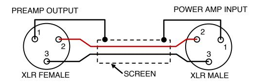
CONVENTIONAL: SCREEN CONNECTED AT BOTH ENDS
