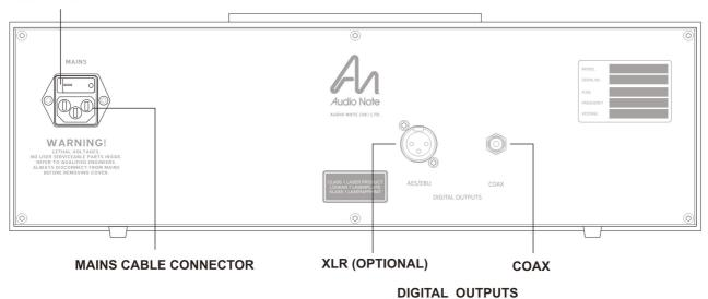
Connectors on the back of CDT Five unit provide a digital output for connection to your DAC via your digital interconnect with RCA connectors. <u>XLR connection is optional</u>, please contact your Audio Note dealer if you require it. Your dealer can advise on suitable type and quality of cable eg: - Audio Note PALLAS or digital SOGON50 are excellent choices.
