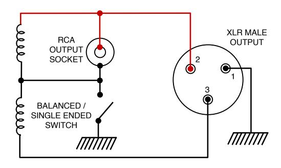
The pin configuration for all Audio Note (UK) XLR / BALANCED connections is as follows: -
