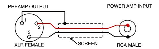
CABLE CONFIGURATION FOR XLR BALANCED PREAMP
