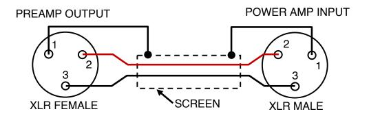
**CONVENTIONAL: SCREEN CONNECTED AT BOTH ENDS**
