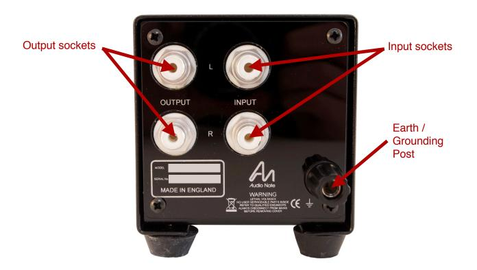
Once located, connect the AN-S3 between your turntable and phonostage input. Connect your tonearm / turntable output cables to the input sockets on the AN-S3, and the output sockets of the AN-S3 to your MM phonostage input. It is important to use good quality, shielded interconnects for all turntable connections; this will help to minimize any noise or hum problems.
