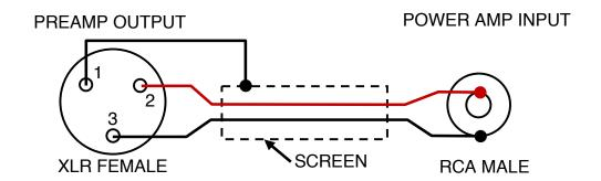
CABLE CONFIGURATION FOR XLR BALANCED PREAMP
