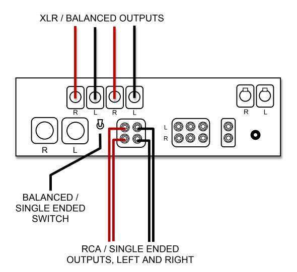
**RCA** The two pairs of RCA / Single Ended outputs are provided for connection to power amplifiers. They are identical, making them suitable for bi-amping.
