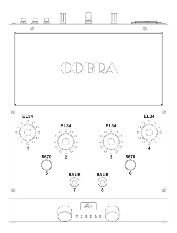
VALVE 1, 2, 3, 4 - EL34 VALVE 5, 6 - 5670 VALVE 7, 8 - 6AU6
