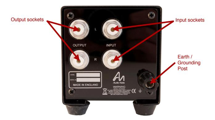
Once located, connect the AN-S4 between your turntable and phonostage input. Connect your tonearm / turntable output cables to the input sockets on the AN-S4, and the output sockets of the AN-S4 to your MM phonostage input. It is important to use good quality, shielded interconnects for all turntable connections; this will help to minimize any noise or hum problems.
