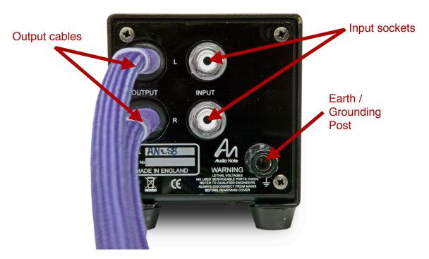
Once located, connect the AN-S8 between your turntable and phonostage input. Connect your tonearm / turntable output cables to the input sockets on the AN-S8, and the output cables of the AN-S8 to your MM phonostage input. It is important to use good quality, shielded interconnects for all turntable connections; this will help to minimize any noise or hum problems.
