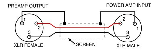
**CONVENTIONAL: SCREEN CONNECTED AT BOTH ENDS**
