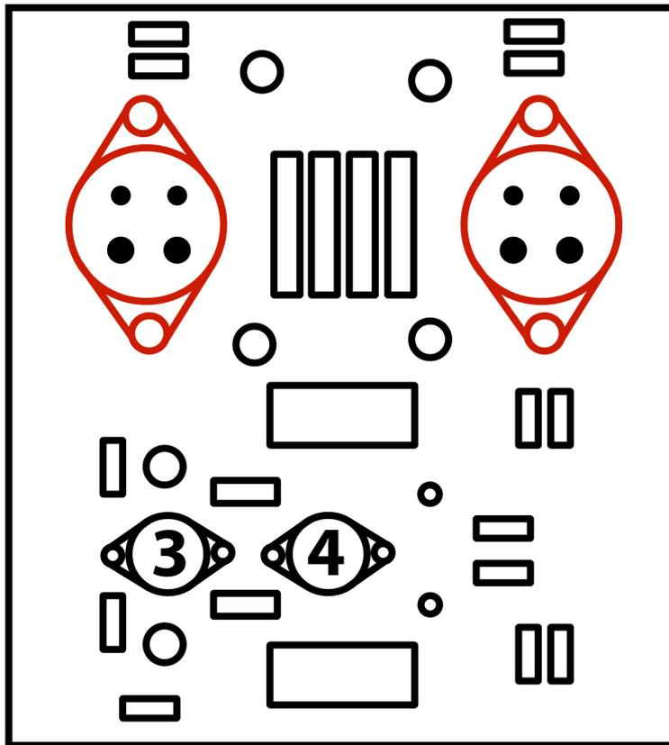
Inspect the bottom of a **300B** valve and the corresponding valve base on the circuit board. You will notice that two of the pins are of a larger diameter than the other two; this is to help ensure that the valve can easily be inserted correctly.
