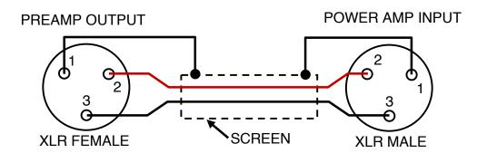
CONVENTIONAL: SCREEN CONNECTED AT BOTH ENDS
