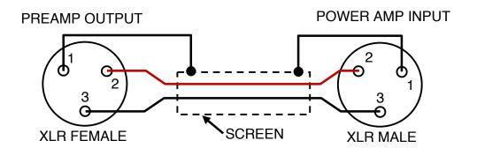
CONVENTIONAL: SCREEN CONNECTED AT BOTH ENDS
