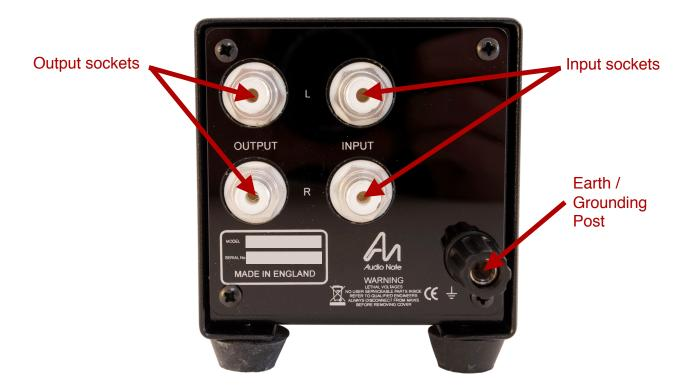
Once located, connect the AN-S5 between your turntable and phonostage input. Connect your tonearm / turntable output cables to the input sockets on the AN-S5, and the output sockets of the AN-S5 to your MM phonostage input. It is important to use good quality, shielded interconnects for all turntable connections; this will help to minimize any noise or hum problems.
