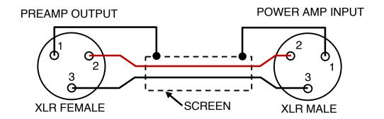
CONVENTIONAL: SCREEN CONNECTED AT BOTH ENDS
