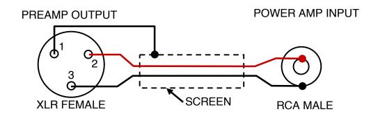
CABLE CONFIGURATION FOR XLR BALANCED PREAMP
