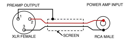
CABLE CONFIGURATION FOR XLR BALANCED PREAMP
