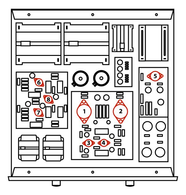
VALVE 1; 300B VALVE 2; 300B VALVE 3; 6463 VALVE 4; CV4068 VALVE 5; 5U4G VALVE 6; 5670 VALVE 7; 5670 VALVE 8; 5670
