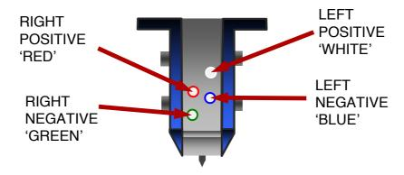
UNDER NO CIRCUMSTANCES SHOULD THE HEAD-SHELL WIRES BE SOLDERED DIRECTLY TO THE CONNECTION PINS OF THE CARTRIDGE BODY. HEAT APPLIED TO THE CONNECTION PINS WILL CAUSE IRREPARABLE DAMAGE.
