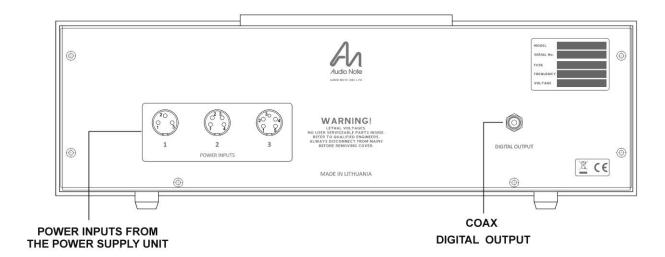
Digital output connector on the back of *CDT Six* unit provide a digital output for connection to your DAC via your digital interconnect with RCA connectors. Your dealer can advise on suitable type and quality of cable eg: - Audio Note digital SOOTTO or Black Pallas both are an excellent choice.
