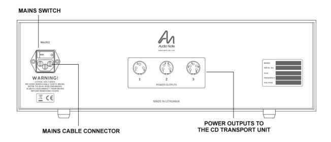
Mains connector on the back of the *CDT Six Force*: An IEC power connector is available for connection to the mains using the supplied mains cable. For further improvement is sound, we recommend to use Audio Note SOGON mains cable.
