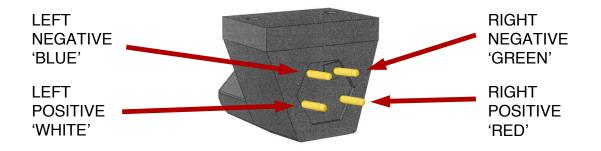
UNDER NO CIRCUMSTANCES SHOULD THE HEAD-SHELL WIRES BE SOLDERED DIRECTLY TO THE CONNECTION PINS OF THE CARTRIDGE BODY. HEAT APPLIED TO THE CONNECTION PINS WILL CAUSE IRREPARABLE DAMAGE.
