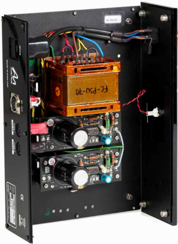
The AN-E includes a power supply (left) and an external crossover (bottom). The open cabinets provide an insight into the finely tuned selection of “sound materials,” which is a tradition with the British: transformers and chokes cast in-house, insulated capacitors, made in-house and custom resistors hand-made in-house, wound on Permalloy board material – absolutely nothing is left to chance here.
