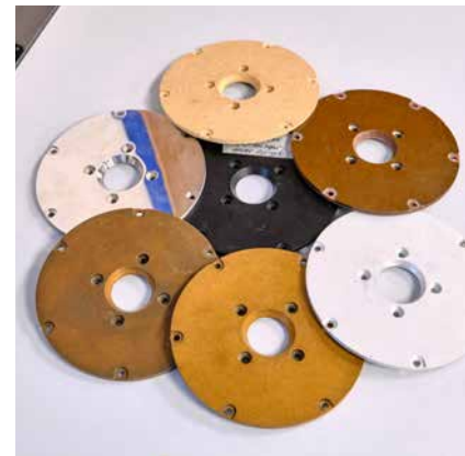
Visiting England: Peter Qvortrup showed us around his company and the in-house production of field coil drivers. The material-obsessed sound tinkerers even tried out several face plate options for the AN-E's tweeter before the ideal "sound metal" was found.
