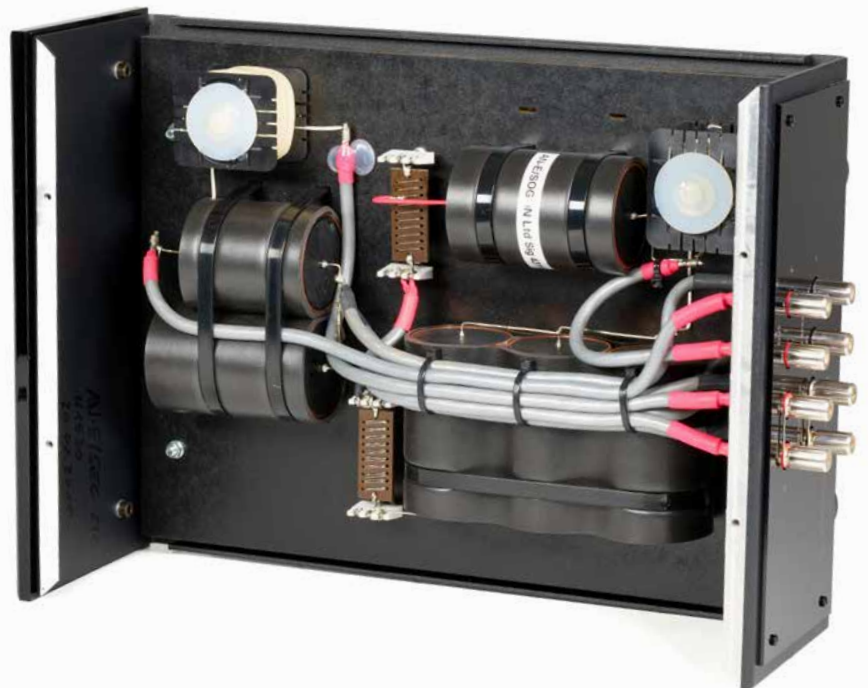
The AN-E includes a power supply (left) and an external crossover (bottom). The open cabinets provide an insight into the finely tuned selection of “sound materials,” which is a tradition with the British: transformers and chokes cast in-house, insulated capacitors, made in-house and custom resistors hand-made in-house, wound on Permalloy board material – absolutely nothing is left to chance here.
