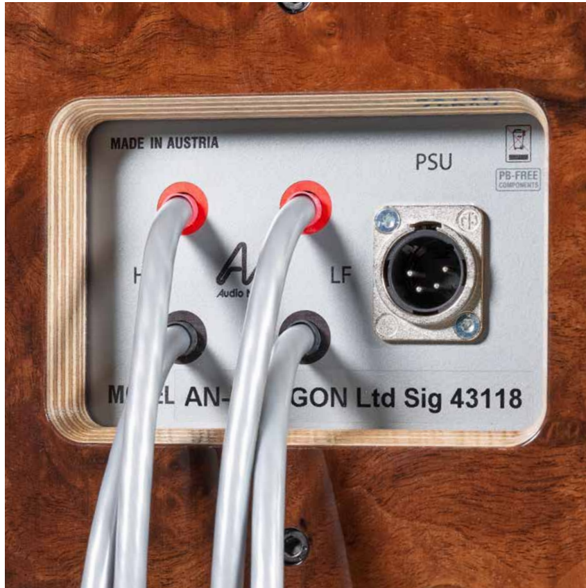
The high-quality speaker cables are permanently fixed to the terminal of the AN-E Ltd. To the right of the access points you can see the four-pin power connection of the power supply unit. The small pictures next to it show the associated cable and the included spikes, which we left in the box during setup. Mounting them only makes sense when you've found the optimum position.
