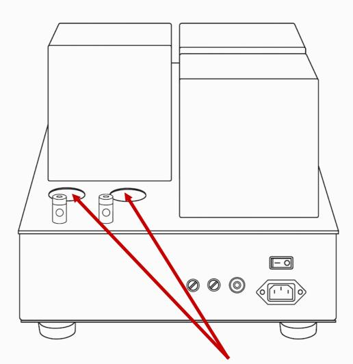
Looking from the back of the amplifier, insert the **5R4WGB** valves into the two empty sockets located on the left, situated between the black rectangular transformer covers and the loudspeaker connection binding posts. Locate the rib on the central pin of the valve and align with the valve base (it can only be inserted one way due to this locating rib) and with gentle but firm pressure insert the valve.
