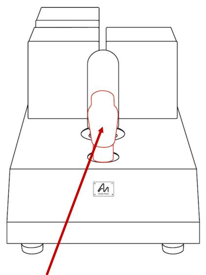
Finally, insert the VT25  $\frac{1}{7}$  10Y into the front socket. The valve can only be inserted one way.
