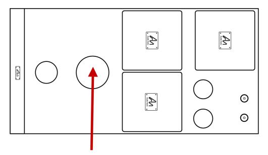
Also examine the large aperture in the top plate of the amplifier, located between the small front valve and the black rectangular transformer covers. This is the insertion points for the 211 valve.
