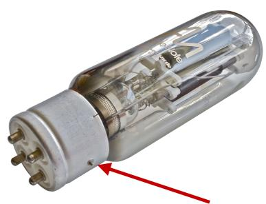
Inspect a 211 valve and you will notice that there is a small 'pin' protruding from one side of the valve base; this locating pin ensures that the valve can only be correctly inserted into the amplifier in one way.
