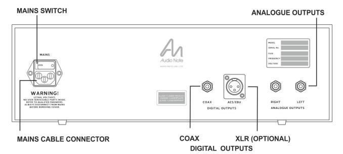
Connectors on the back of *CD3.1x/ll* unit provide digital and analogue outputs.
