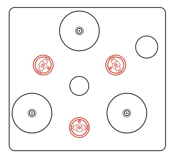
Place the sub-chassis on the base / motor unit. *IT IS ESSENTAIL THAT THE SUSPENSION TOWERS ARE CORRECTLY ALIGNED WITH THE PILLARS / TUBES ON THE UNDERSIDE OF THE SUB-CHASSIS*:
