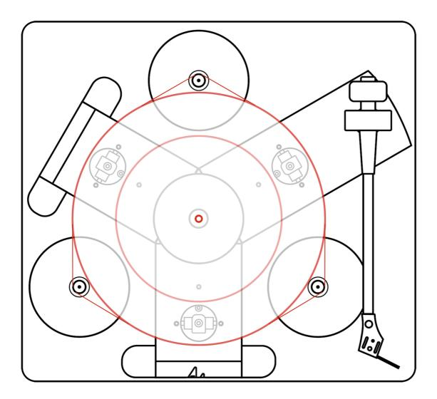
The belt should settle at the centre of the platter's edge, all the way around the circumference of the platter. If this is the case once the belt and platter have been installed, then simply check that the platter is level with a spirit level (both from front to back and left to right) and if so, the suspension set up is complete and you can install the cartridge.
