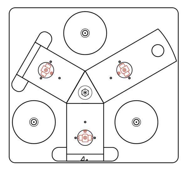
The ends of the white suspension bars (shown below in RED) must be located correctly in the two notches, located on either side of the bottom of each of the three suspension tower pillars / tubes, which are on the underside of the sub-chassis. *CHECK THAT THIS IS CORRECT FOR ALL THREE SUSPENSION TOWERS*:
