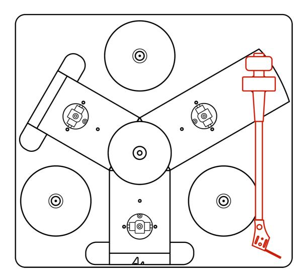
Once the tonearm has been installed, final adjustment of the suspension can be performed. (The suspension is adjusted at the factory, but this setup can move during transit).
