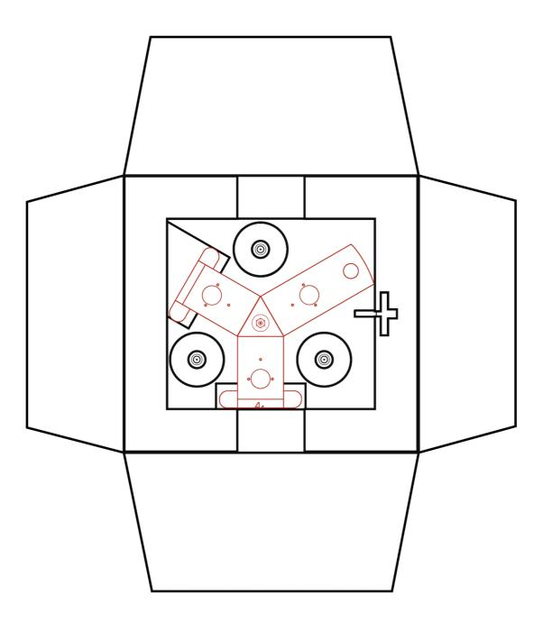
Locate and remove the sub platter / bearing (shown in RED):
