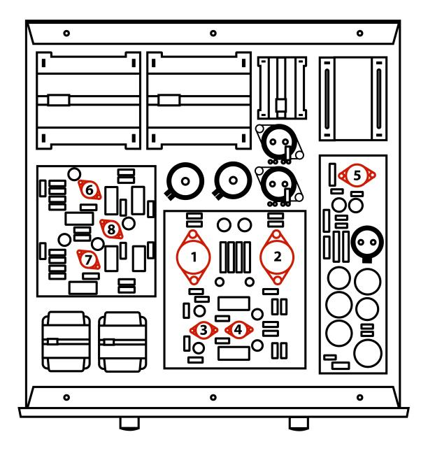
VALVE 1; 300B VALVE 2; 300B VALVE 3; 6463 VALVE 4; CV4068 VALVE 5; 5U4GB VALVE 6; 5670 VALVE 7; 5670 VALVE 8; 5670
