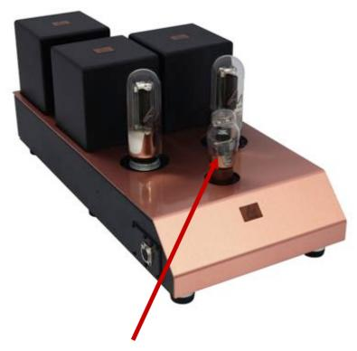
Finally, insert the VT25 / 10Y into the front socket. The valve can only be inserted one way.
