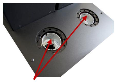
Also examine the two large apertures in the top plate of the amplifier, located between the small front valve and the black rectangular transformer covers. These are the insertion points for the 211 valves.
