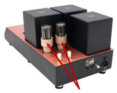
Looking from the back of the amplifier, insert the **5R4WGB** valves into the two empty sockets located on the left, situated between the black rectangular transformer covers and the loudspeaker connection binding posts. Locate the rib on the central pin of the valve and align with the valve base (it can only be inserted one way due to this locating rib) and with gentle but firm pressure insert the valve.
