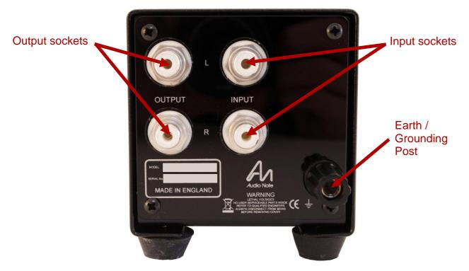
Once located, connect the AN-S5 between your turntable and phonostage input. Connect your tonearm / turntable output cables to the input sockets on the AN-S5, and the output sockets of the AN-S5 to your MM phonostage input. It is important to use good quality, shielded interconnects for all turntable connections; this will help to minimize any noise or hum problems.
