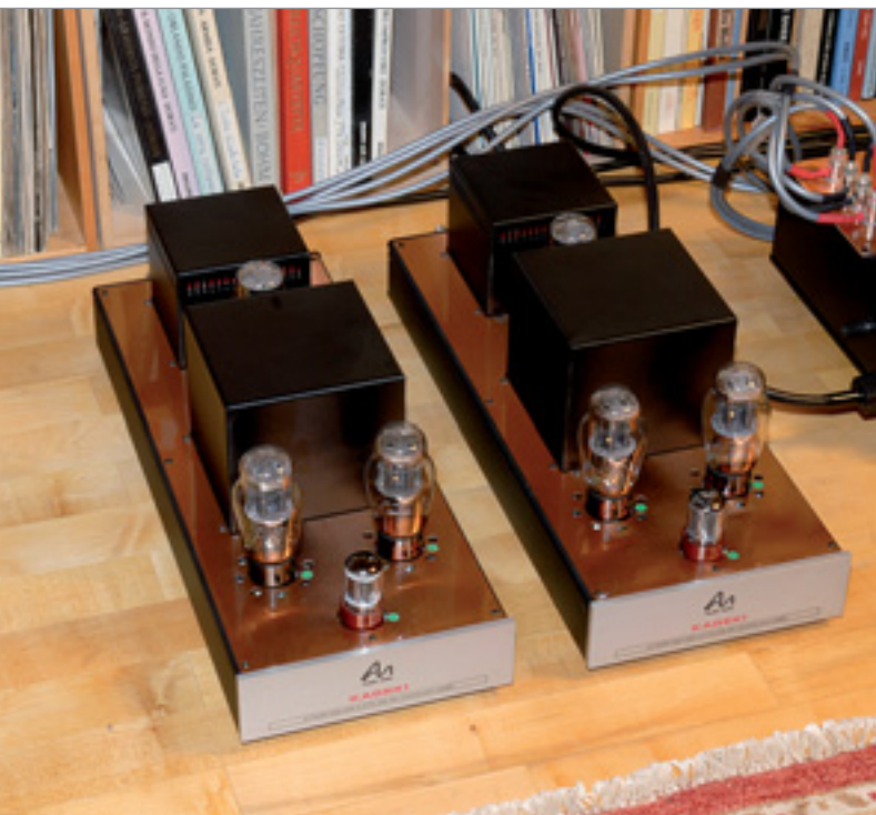
They don't necessarily need a special platform to perform: Kageki monos with 2A3 and pure silver output transformers
