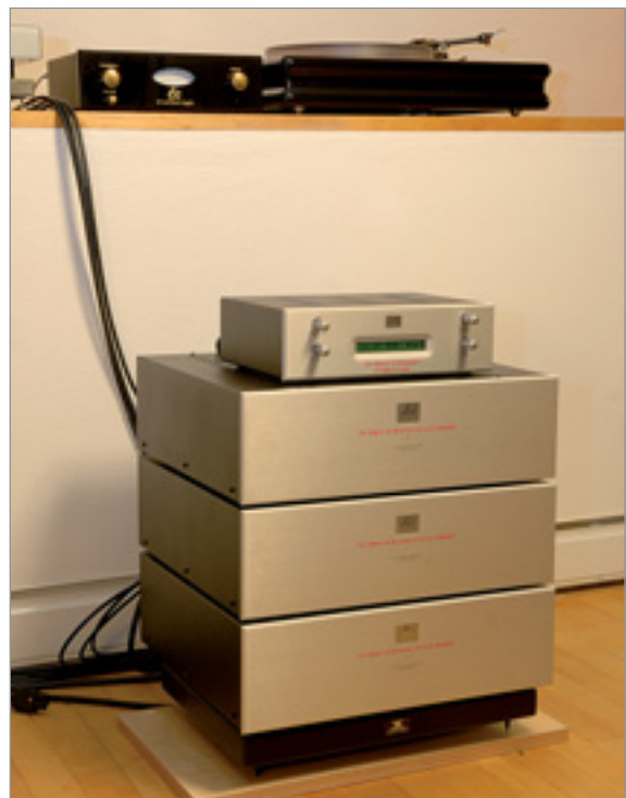
Top: TT3 Reference with power supply for the IO Ltd cartridge. Below: Control device and power supplies for the three TT3 motors
