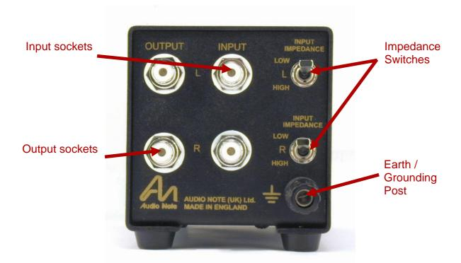
Once located, connect the AN-S2 between your turntable and phonostage input. Connect your tonearm / turntable output cables to the input sockets on the AN-S2, and the output sockets of the AN-S2 to your MM phonostage input. It is important to use good quality, shielded interconnects for all turntable connections; this will help to minimize any noise or hum problems.
