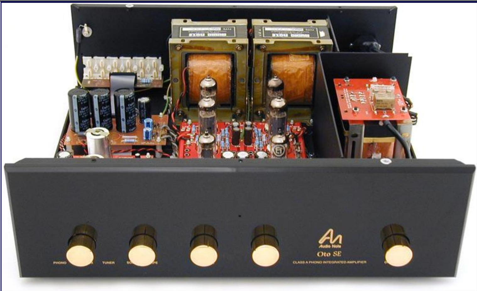
Indeed, in a real sense the OTO is a different animal than a lot of integrateds that are designed as a cost-cutting measure at the design stage. This amplifier is in fact, dedicated preamp and power amp separates sharing one bigger box. Indeed, if you look at the innards of the M1 and P1, you can see very similar layouts.
