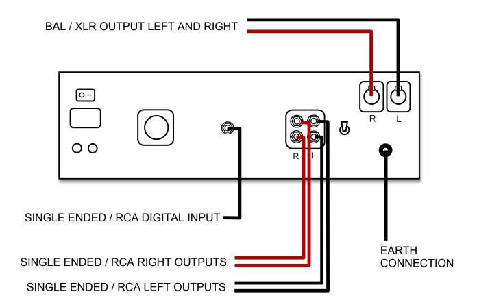
**RCA** The two pairs of RCA / Single Ended outputs are identical, and are for connection to a pre amplifier or recording device.
