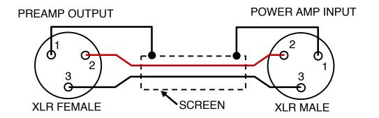
**CONVENTIONAL: SCREEN CONNECTED AT BOTH ENDS**
